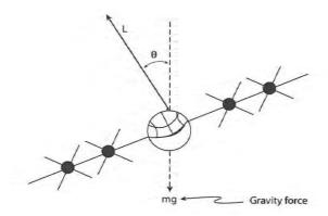
For a semi-vertical angle of  $\theta$  and velocity  $\nu$ , show that the radius of the turning circle, R
